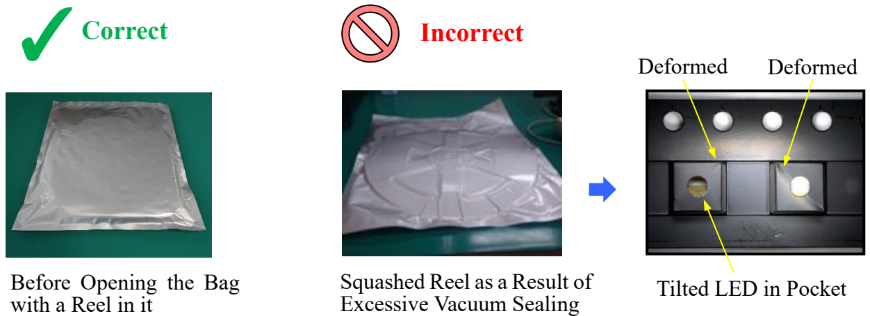
Figure 4. Correct/Incorrect Examples for Embossed Carrier Tape after Vacuum Sealing
