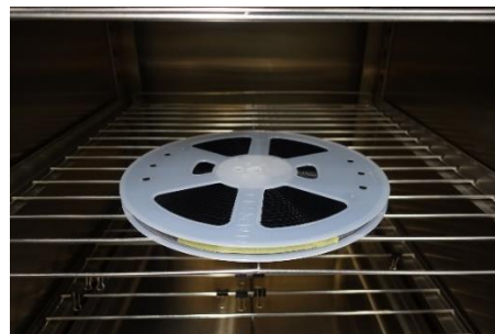
Figure 3. Example for Baking the LEDs
